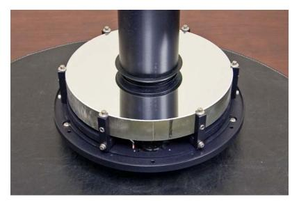
The completed primary mirror assembly is shown above with the primary mirror alignment mark in the up position. Make sure that all mirror clips are at the proper height and completely secured before handling the assembly. The back plate handles provide a safe way of handling the assembly.
