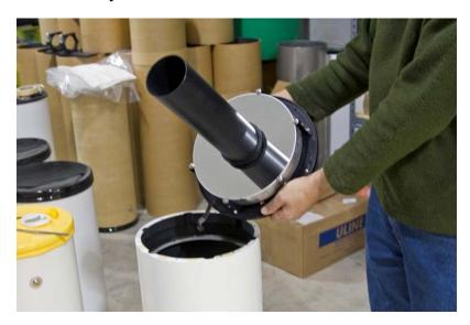
The primary mirror assembly is best installed with the OTA standing on end as shown. It is highly recommended that this procedure be performed by two persons. Care should be taken not to damage the primary mirror or drop something onto the secondary mirror. The primary mirror baffle is inserted into the OTA first and the assembly is carefully lowered.
