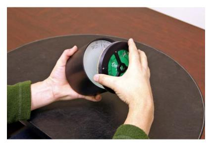
The secondary mirror back plate may now be screwed into place. Do not force this as the threads are fine and can easily be cross-threaded. If the back plate does not thread easily, inspect the threads for debris and clean as necessary.
