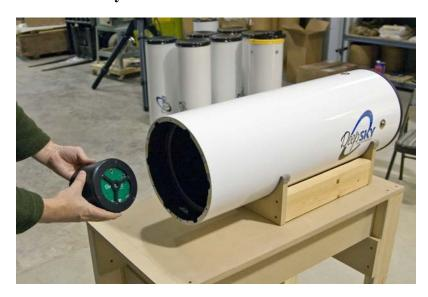
The secondary mirror assembly may now be installed into the OTA. It is inserted into the tube from the rear.
