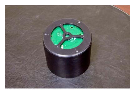
The back plate should only be tightened enough so that the secondary mirror does not move within the cell. Over tightening may result in pinching the secondary mirror and distorting the telescope image.
