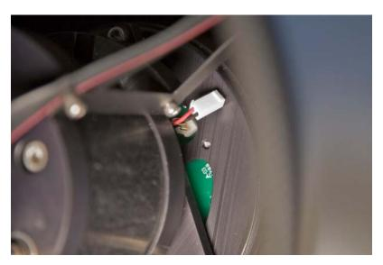
The secondary dew heater connects to the secondary focuser assembly with a two position connector as shown. The connector has a positive latch to help stay connected but will pull apart if something should bind to avoid permanent damage.
