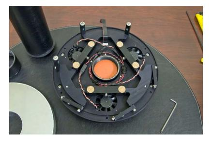
The primary mirror cell is a six point floatation cell consisting of three rockers. The primary mirror is held in place and centered by six mirror clips. Three of these clips are shown in there final position while three are loose. The cooling fan wiring is secured to the back plate with silicon adhesive. A single ribbon cable connects the back plate to the OTA body and provides control of the secondary focuser and dew heater.
