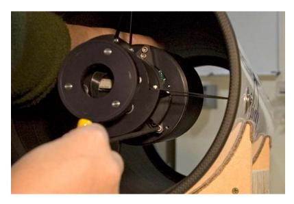
All three secondary mirror collimation screws should be secured in this fashion. The secondary mirror collimation set screws are generally not touched so that the assembly is returned to roughly the same position it was in before it was removed.
