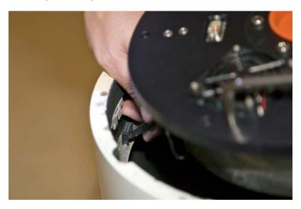
While holding the primary mirror assembly just above the OTA, the ribbon cable connector must be connected to the mating connector inside the OTA. The ribbon cable is just long enough accomplish this.
