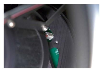
Here is the dew heater connector shown in place.
