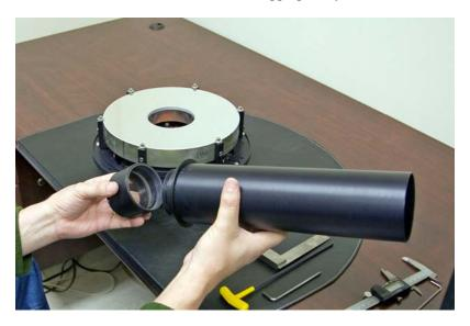
The corrector/field flattener cell (RC10C) or spacer (RC10) firmly screws into the rear of the primary mirror baffle tube.
