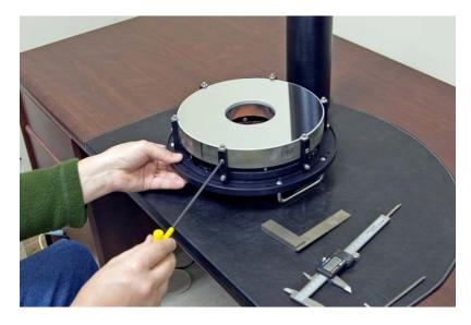
Any adjustments to the set screws should be made with an appropriately sized hex wrench.
