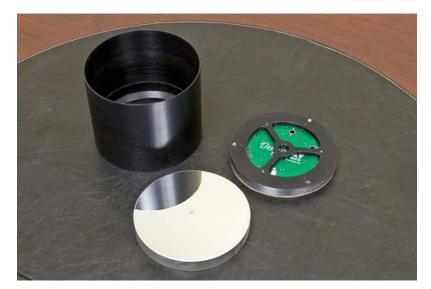
The secondary mirror assembly consists of the secondary mirror, secondary baffle and secondary back plate. The secondary back plate contains the secondary dew heater which is simply an array of resistors.
