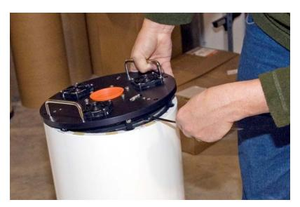
The excess cable must be stowed behind the primary mirror. This is done by slowly lowering the primary mirror assembly into place. The side nearest the connector (bottom) should be held away from the OTA and a flat thin object (a steel ruler in the picture above) is used to push the excess cable behind the primary mirror. The back plate may then be lowered into position.
