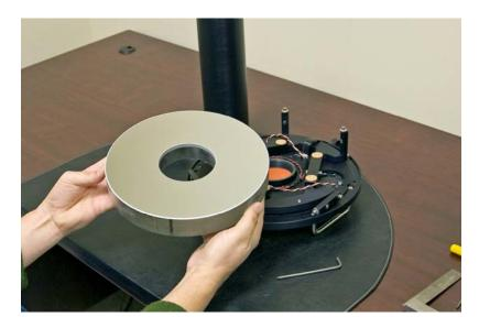
The primary mirror should be handled with care to avoid damage and contact with the optical surface.
