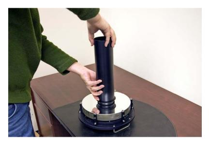
This assembly then screws into the back plate adapter. Be very careful not to damage the primary mirror.
