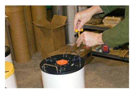
The back plate mounting holes should be aligned with the corresponding holes in the OTA. Make sure the back plate is completely seated and nothing is being pinched. The fastener screws should screw with little or no force if the holes are properly aligned. Do not force these screws as this may be an indication that something is not right.
