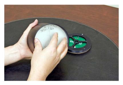
Once the secondary mirror is fully seated, be careful to keep the secondary mirror baffle upright so the secondary mirror does not fall out.
