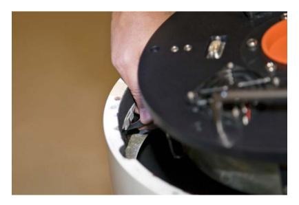
This is how the cable looks after the connection is made. Once connected, be careful not to pull against the cable.
