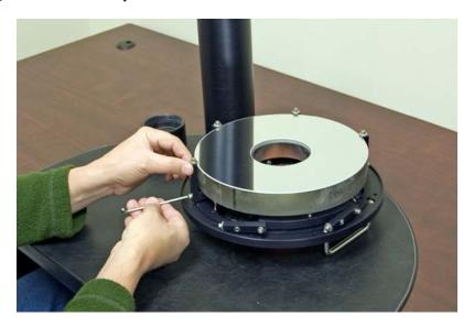
Once the primary mirror is in place, the mirror clips may be replaced. This is done with a properly sized hex wrench.
