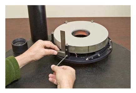
The mirror clips should be square to the back plate.
