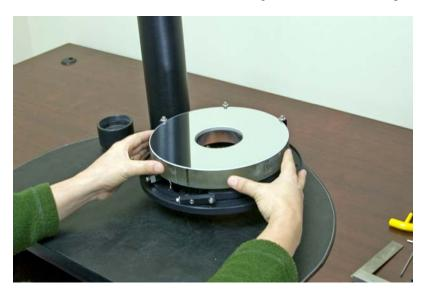
Carefully place the primary mirror on the primary mirror cell. It should be roughly centered. If the mirror was removed for cleaning by loosening three of the mirror clips, it may be returned to its previous position using the other three clips as a reference.
