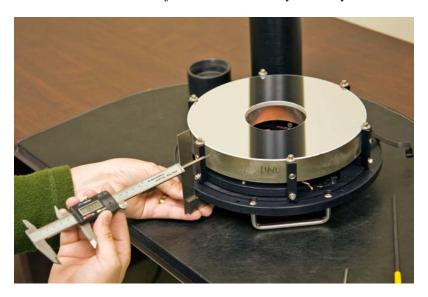
The mirror should be centered in the back plate. If required, the set screws may be adjusted to accomplish this. One procedure using calipers and a square is shown above. This generally works well as the mirror's outer diameter is fairly round. The mirror is centered when opposite measurements are within 0.01 inches or so. Misalignment by significantly more than this can lead to astigmatism.
