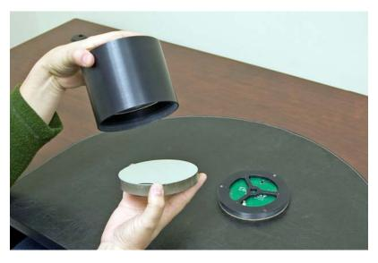
Insert the secondary mirror into the secondary mirror baffle being careful not to damage the secondary mirror. The fit will be fairly tight so the secondary mirror must be kept square to the secondary baffle. Make sure the secondary mirror seats completely and does not get wedged.
