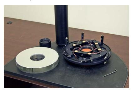
The primary mirror assembly consists of the OTA back plate, primary mirror, mirror cell and clips, primary mirror baffle and corrector/field flattener (RC10C) or spacer (RC10).
