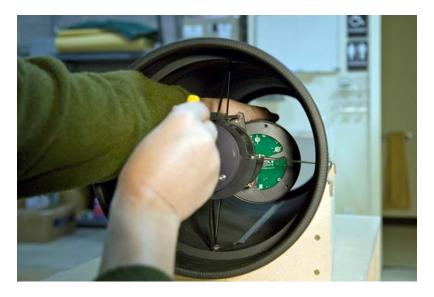
The secondary focuser assembly is not intended to be serviceable in general. In order to install the secondary mirror assembly, you must reach between the spider vanes and lift the assembly into place. Make sure the top of the assembly is installed upwards as shown. A long handled hex wrench should be used to secure the assembly.
